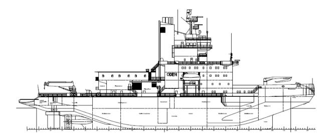
Oden is one of five icebreakers operated by the Swedish Maritime Administration. The vessel is designed for escort, ice-breaking and for Arctic research operations with non-limited trade areas. The icebreaker is also a research platform with a very flexible layout and can carry scientific equipment, container/van labs, frozen storage and equipment for geological sampling, oceanography, meteorology and other disciplines.
