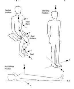
x-axis:  $W_d$  k=1,4 y-axis:  $W_d$  k=1,4 z-axis:  $W_k$  k=1,0
